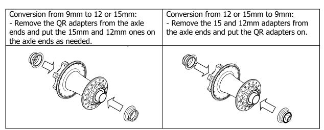
a) Remove the axle end mounted on the hub (QR or 12x142). If needed, pull strongly to take it away, it is due to the O-ring which holds in place the axle end.
