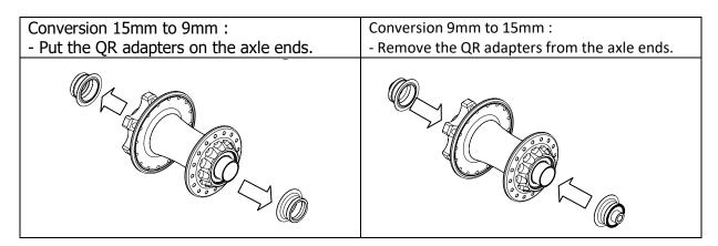
a) Remove the axle end mounted on the hub (QR or 12x142). If needed, pull strongly to take it away, it is due to the O-ring which holds in place the axle end.
